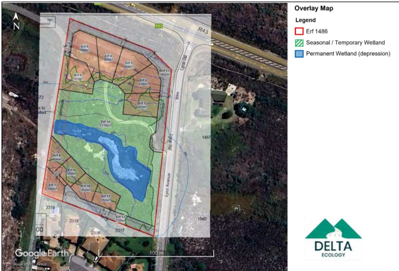
Figure 7-1: Preferred Layout (Alternative 4) for the site overlain with the delineated UVBW onsite. This preferred layout has minimal wetland encroachment.
