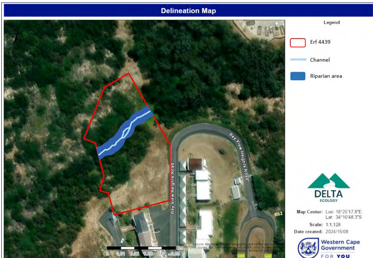
Figure 5-7: Delineation of the non-perennial drainage line, i.e. the active channel and the riparian area.
