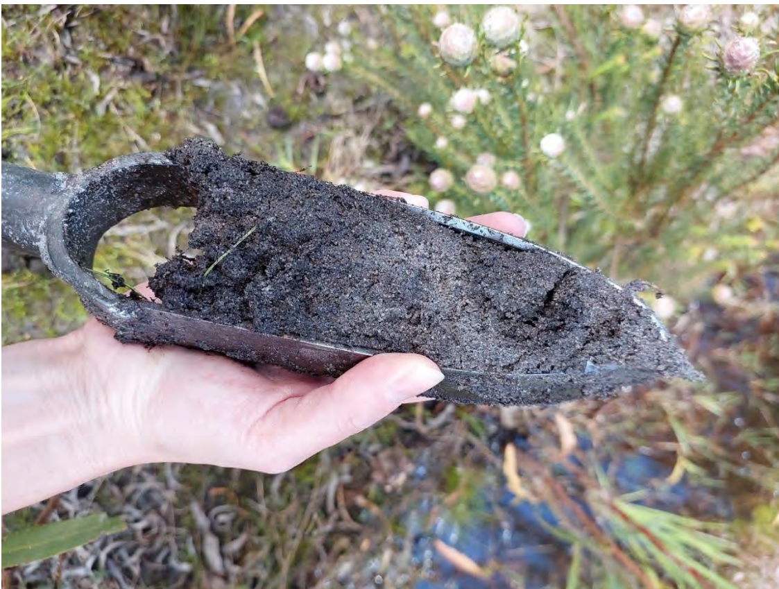
Figure 5-10: Soil sample illustrating organic surface layer & gleying typical of the permanent/seasonal wetland zone.
