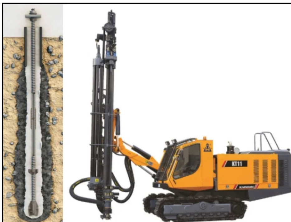
Figure 3. Self Drilling Anchor pile and installing rig. Courtesy Mike Hurworth, MH&A Consulting Engineers.
