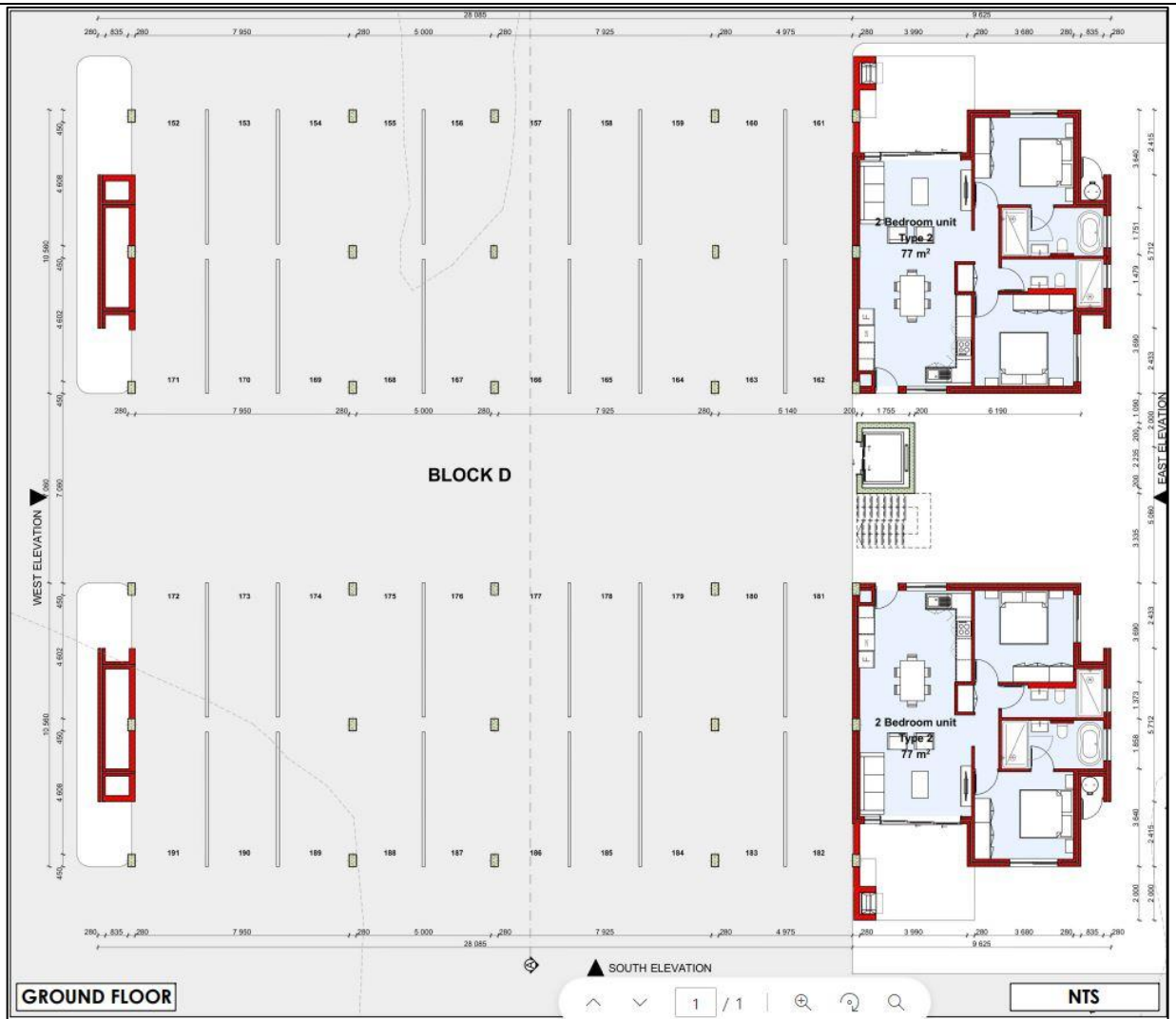
Figure 2: Ground floor layout: 2 flats with 2 bedroom each, along with the parking area situated on the ground floor.
