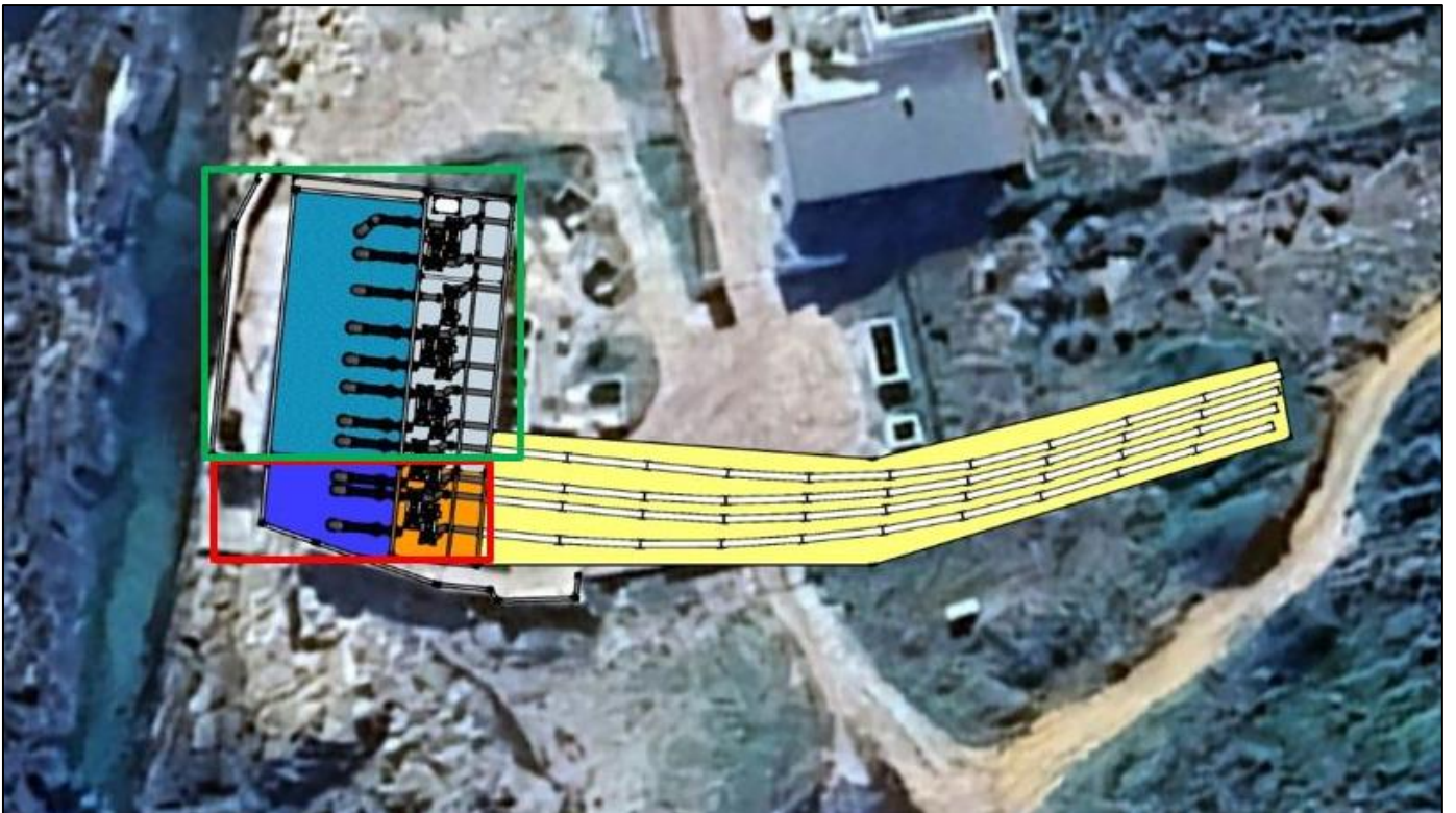
Figure 3a, 3b: View of the existing pumphouse (green) and the area outlined in red, which is proposed for expansion to accommodate the installation of new pipelines. One pipeline will be integrated into the existing pumphouse infrastructure, as illustrated.
