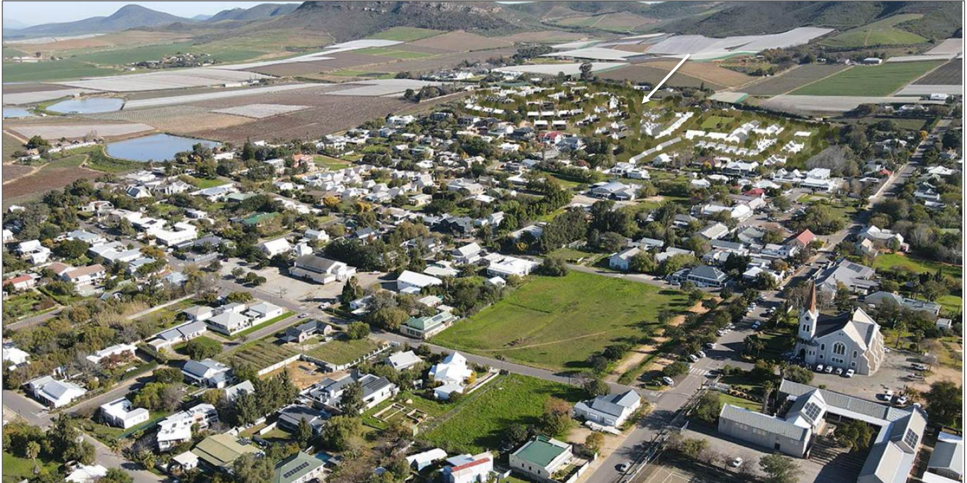
Figure 121: Photomontage of the proposed neighbourhood using the urban design recommendations to create a new development that sits comfortably on the hill, nestled by banks of trees. The scale of houses on the hill is broken horizontally (Plinth, body, roof) to mitigate scale. The lines of trees in the new neighbourhood ties into the existing town treescape and grid
