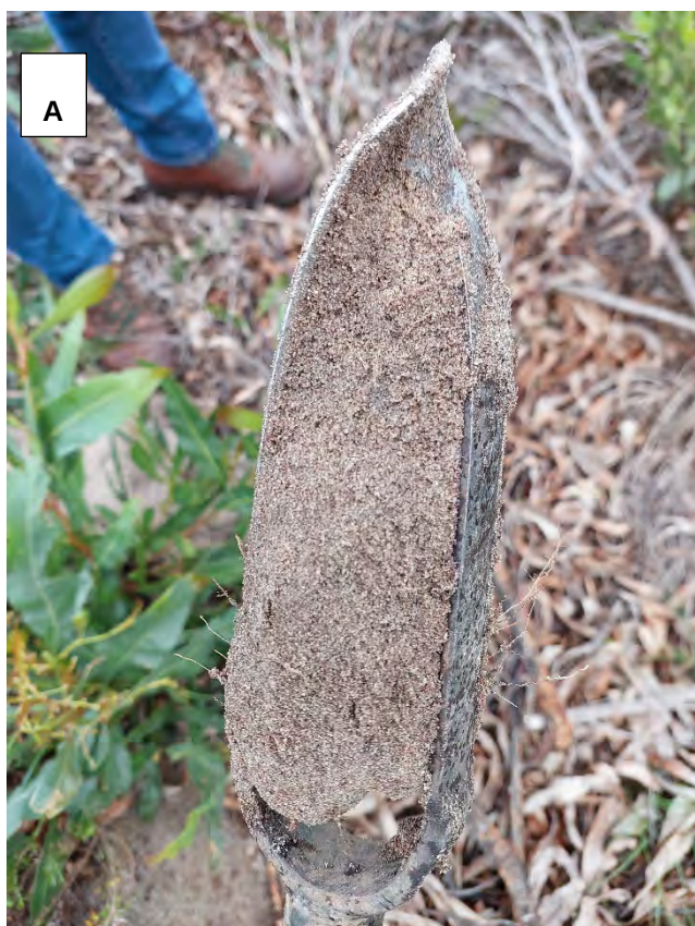
Figure 5-8: A) Near-surface soil sample, showing typical terrestrial soil conditions within the study area. Terrestrial soils within the study area are sandy, characterised by a uniform grey – brown colour, with no mottling, gleying or organic matter visible. B) Near-surface soil sample, taken within a wet area; darker chroma observed.
