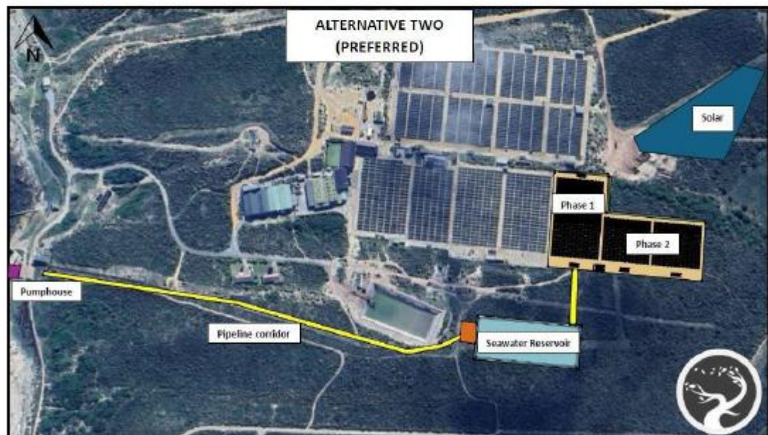
Figure 1: Preferred layout for the Pre-Application Basic Assessment Report. Note the small extent of the solar array relative to the existing structures and relevant landmarks.
