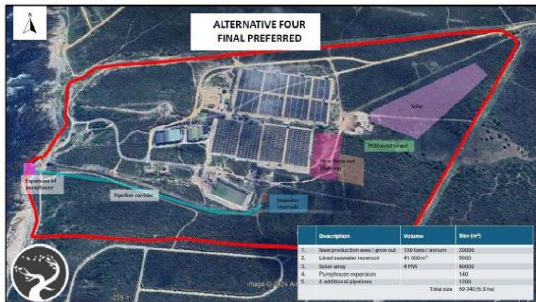
Figure 2: Preferred layout for the Draft Basic Assessment Report. Note the large extent of the solar array relative to the existing structures and relevant landmarks.
