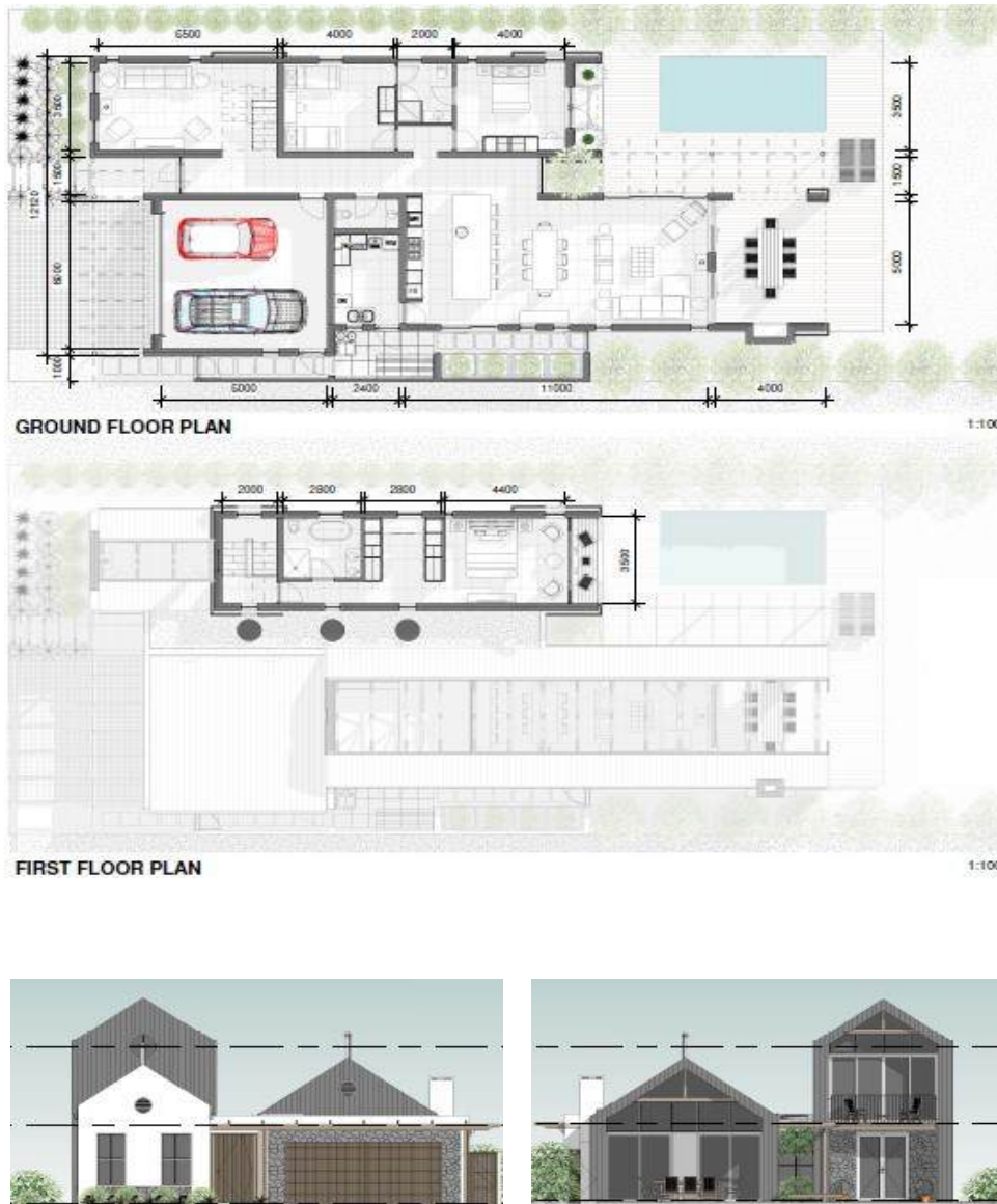
Figure 14. Sample drawings – Plan, elevations and 3D studies for a 3-bedroom house - 'Barn Type 3' (Source: CSA Architecture)
