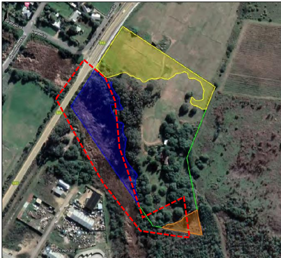
Figure 2. Wetlands on Erf 438, Stanford. Development over the highly degraded hillslope seep wetland indicated in yellow is permitted but a 32m buffer demarcating a Regulated Area is required around the UVB wetlands indicated in blue and orange.
