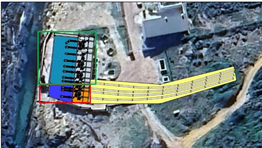
Figure 3-2: View of the existing pumphouse (green) and the area outlined in red, which is proposed for expansion to accommodate the installation of new pipelines. One pipeline will be integrated into the existing pumphouse infrastructure, as illustrated.
