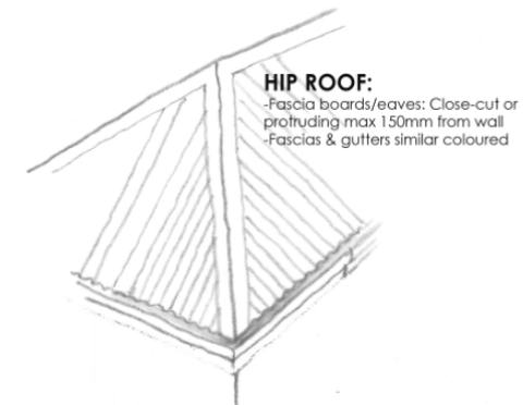
PRIMARY BUILDING ROOF ARTICULATION
