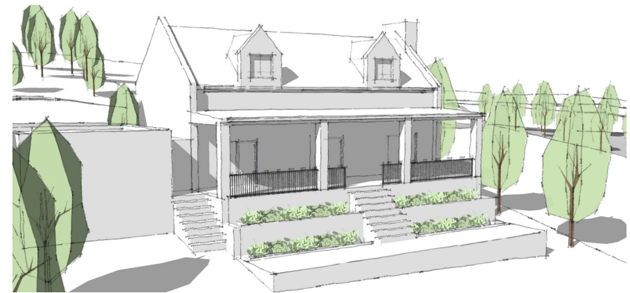
TYPICAL VERANDAH & PITCHED ROOF DORMER COMPOSITION
