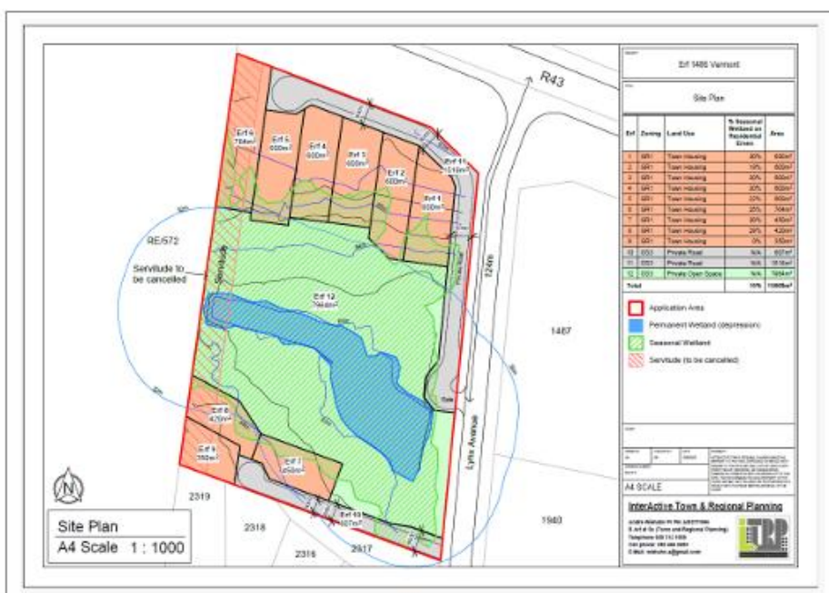
Figure 2. Site development plan (Revision 20D) presented in the Final Basic Assessment Report as Appendix B3 wherein the residential erven encroach into the delineated wetland, and which is not supported by CapeNature.
