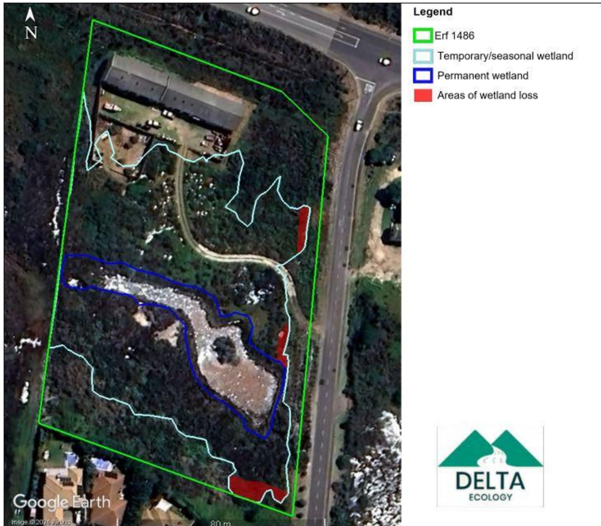
Figure 2. UVB wetland on Erf 1486, Vermont. The development of access roads over the seasonal/temporal zone of the wetland area indicated in red is permitted. The proposed development will result in 0,024 ha of wetland loss, this leaves the remnant 0,876 ha of the UVB wetland available to be used as an offset for the development activities.
